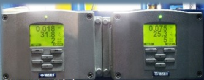
Hygrometer - Vaisala Water content testing result after treating by NSH VFD
